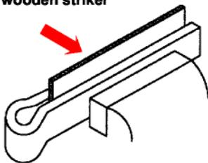
To bend an edge to 90° on a sheet of metal that is larger than the jaws of the vice, **folding bars** can be used to hold the sheet.
